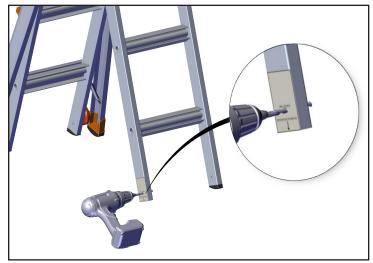
9. To ensure proper hole alignment of outer and inner faces of the rail, you must drill straight through, or drill in from each side of the rail, using the templates.
