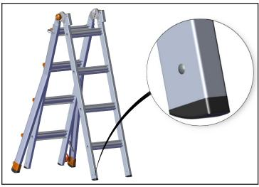
3. If applicable, locate the rivet that is holding the inner foot in place. Ready a drill with a 3/16" bit. If there is no rivet, proceed to step 7.
