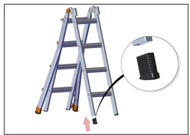
10. Insert the new foot, making sure the thicker side goes towards the outside of the ladder. Then see fastener instructions on the next page.
