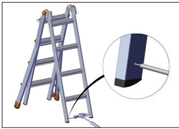
6. Using a hammer and 3/16" punch, completely remove and discard the rivet. Take care not to damage the rail.
