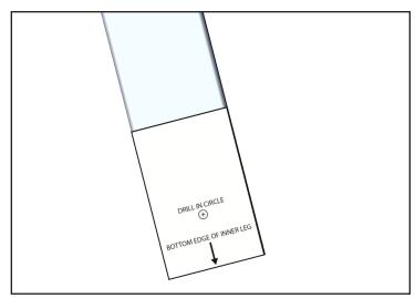
8. If there are no pre-existing rivet holes in your ladder, cut out and align the template at the bottom of the rail, and tape it in place.
