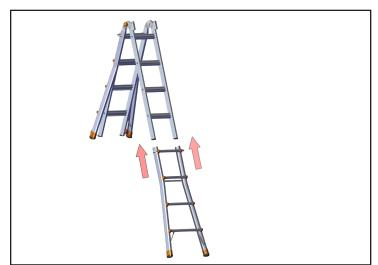
15. Reinstall the outer assembly onto the inner assembly. Make sure the ladder is completely stable before returning it to service.
