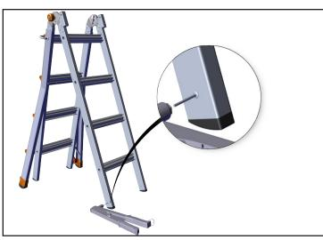
14. Set with a rivet gun. The rivet will expand and flare out, holding the inner foot snugly in place. Repeat this process on the remaining feet. Then proceed to step 15.
