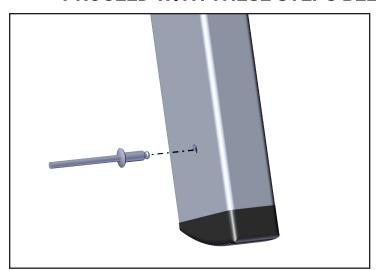
13. Align and insert rivet into the hole at the base of the inner assembly. Only one pop rivet per foot is needed.
