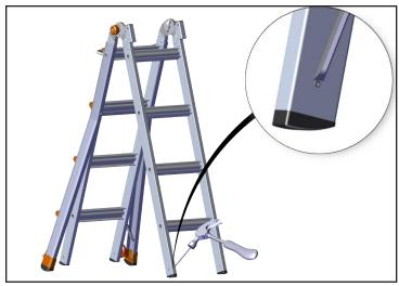
5. If necessary, use a hammer and chisel to remove any remaining clinch material. Take care not to damage the rail.
