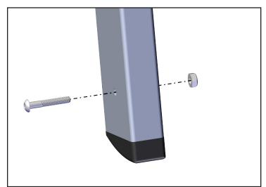
11. Using a 1/8" Allen Wrench and 3/8" wrench, secure the fasteners with the bolt head placed on the outside of the rail and the nut on the inside of the rail.
